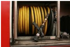
High pressure hose reels are quick, simple, easy, light & fed from an integral water tank.
